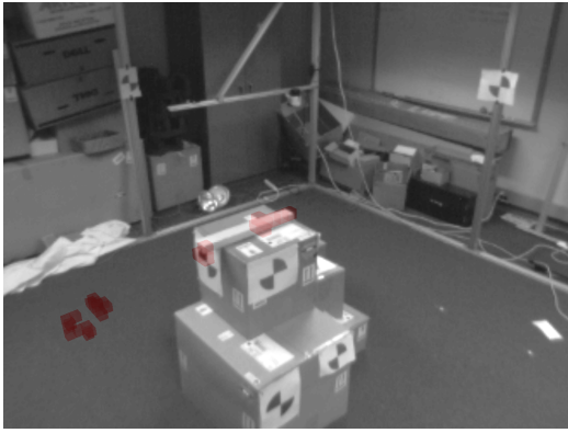
Fig. 6. Foreground occupancy for small object test, using thresholded subtraction and t_f = 0.73 .
