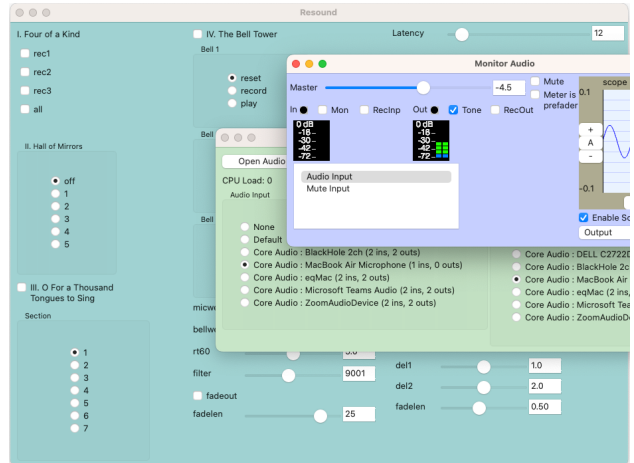
Figure 5. An Arco implementation of “Resound” for trumpet and interactive computer. Control and interface are implemented in the Serpent scripting language. Arco is linked to Serpent as a library.
