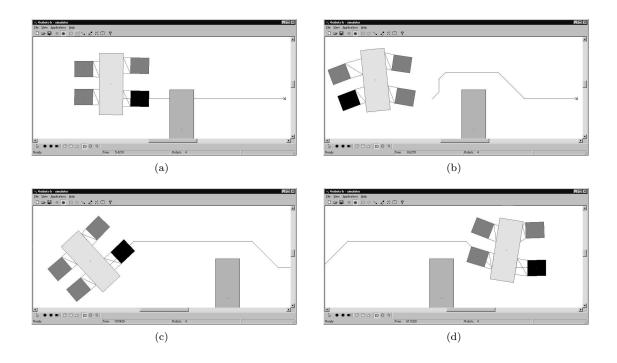
Figure 5: Leadership resignation with four non-holonomic robots transporting an object.
