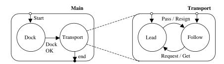
Figure 3: Possible roles in the execution of a cooperative manipulation task. Note that the Transport role is in fact composed by the Lead and Follow roles.
