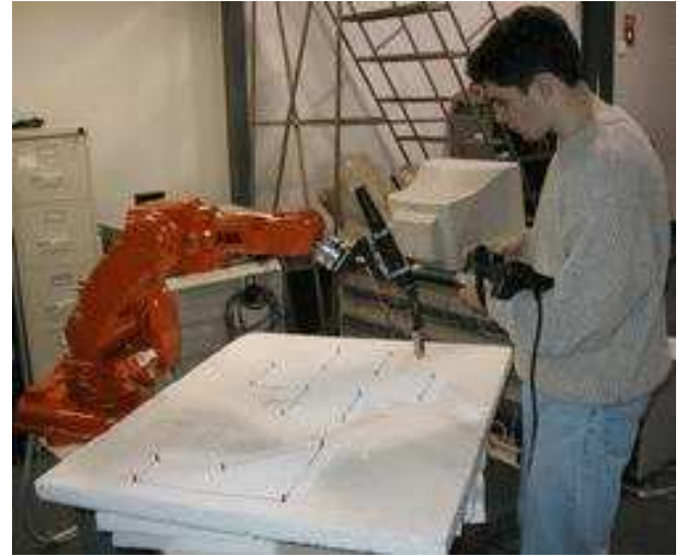
Figure 5: Creating waypoints for the patterns in Figure 4 with an ABB IRB140.
