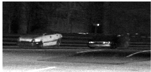
Figure 7. A dark vehicle on the right of the laser image has a similar intensity to the surrounding pixels, except for very strong reflections off the headlights. The white vehicle is more easily detectable.
