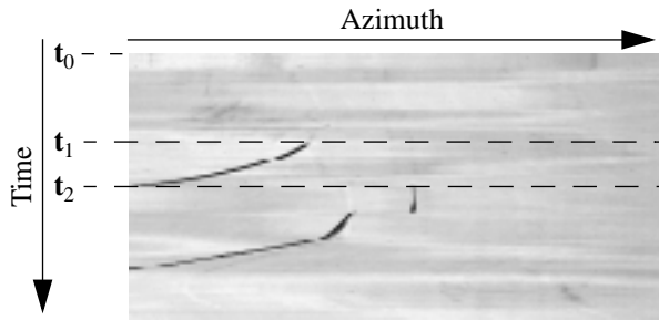
Figure 2. A series of single-line (1-D) laser reflectance scans taken from a moving vehicle (reflectance has been scaled and inverted for better printing). Time t=0 is at the top of the image. Dark spots correspond to obstacles. The vehicle passes two lamp posts on the left (the dark curves), and approaches a cinder block in the center (25 to 30 meters away).
