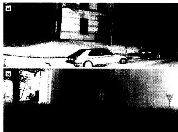
Fig. 2: Images of the laser radar (section: azimuth 60°, elevation 30°) a) Reflectance image b) Range Image
