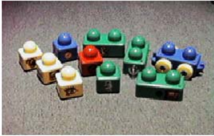
Figure 8. Electronic Blocks: the three sensing blocks are pictured on the left, the logic blocks in the middle, and the action blocks on the right.
