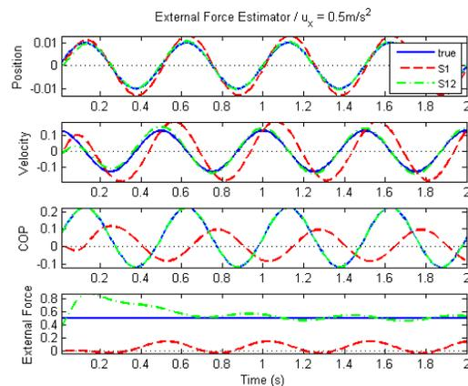
Fig. 7. State estimation performance with unknown external force (D2) comparing position-only measurement (S1) with position and COP measurement (S12). The external force (with a true value of  $u_x = 0.5\text{m/s}^2$ ) is added as an additional state variable in the process model.
