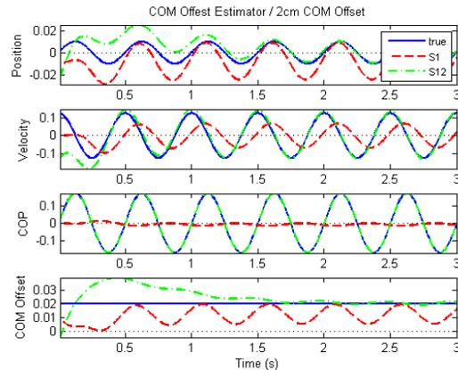
Fig. 6. State estimation performance with unknown COM offset (D1) comparing position-only measurement (S1) with position and COP measurement (S12). The COM offset (with a true value of  $\Delta x = 0.02\text{m}$ ) is added as an additional state variable in the process model.
