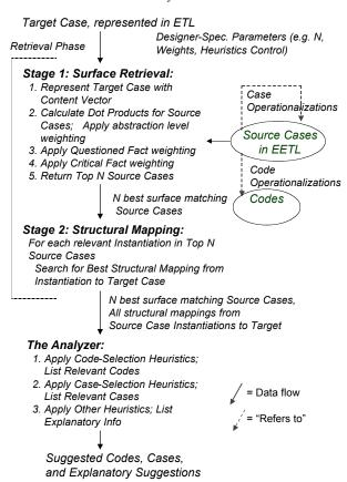
Figure 5: SIROCCO's Algorithm
