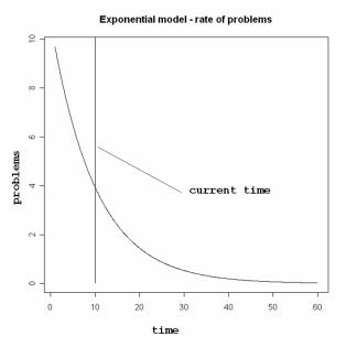
Figure 2. Failure intensity function for the exponential model
